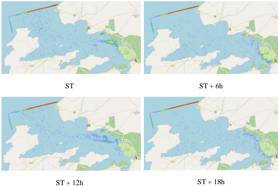
Figure 4.11: Spatial distribution of particles in Kilmakilloge Harbour every 6 hours, ST denotes the spring tide on the 28 th February 2017 at 00h:00mn:00s (i.e after 21 days since release).
